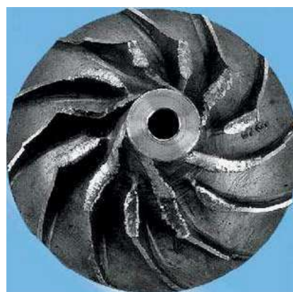
Figure 1. Compressor wheel damaged by a foreign object
