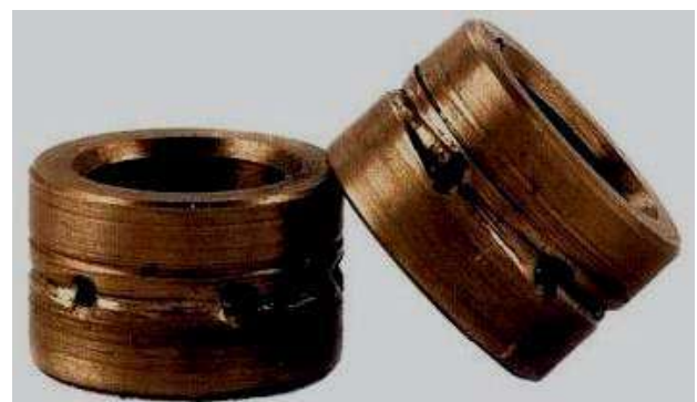
Figure 8. Radial bearings damaged by dirty oil
