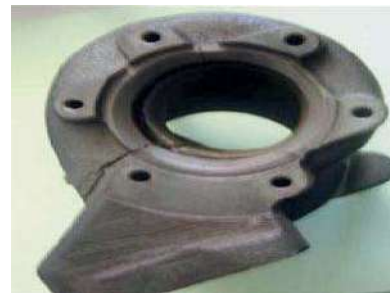
Figure 12. Effect of high temperature on the turbocharger rotor
