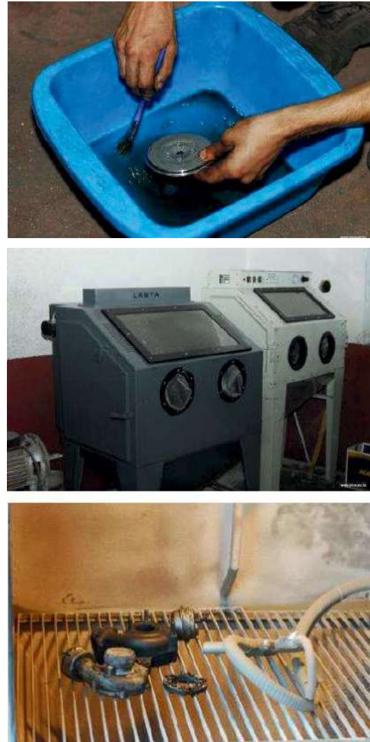
Figure 15. Cleaning, degreasing and sandblasting [1]
