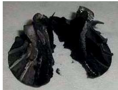
Figure 11. Typical fracture of the turbocharger impeller
