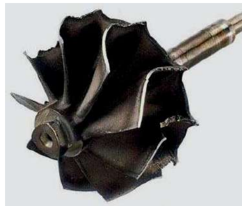
Figure 5. Rotor damaged by foreign objects
